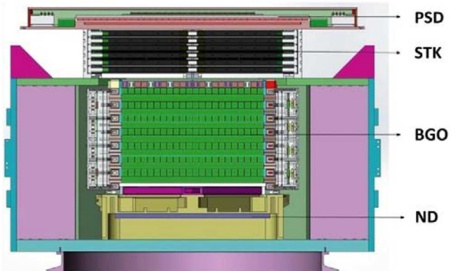
Fig. 1. Architecture of DAMPE payloads.
