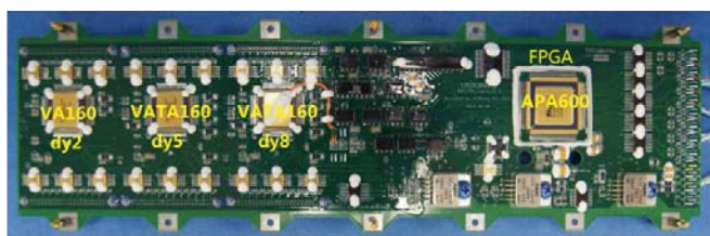
Fig. 17. Photograph of the QM FEE board (Type A).
