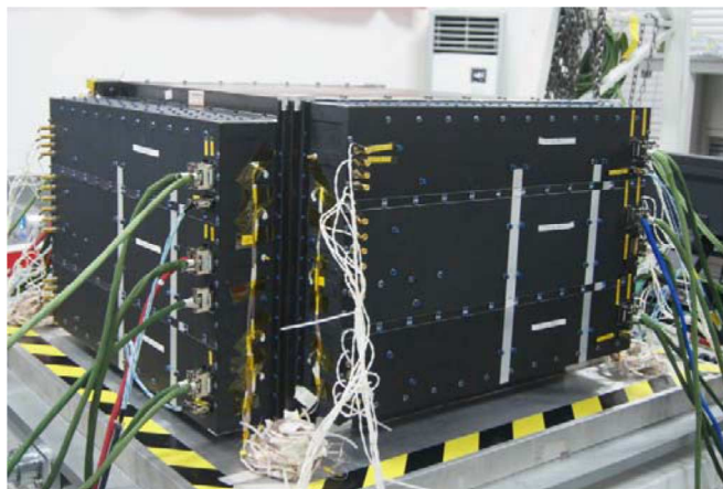
Fig. 18. Photograph of the BGO calorimeter qualification model after assembly.
